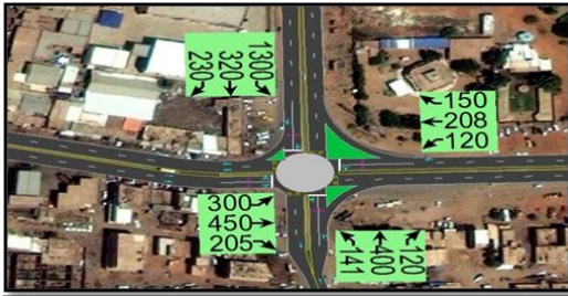
Fig. 8: Shows the number of vehicles at each direction (Source: Researchers, used: traffic simulation)
